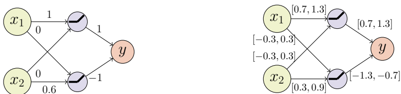
Figure 8: (a) The model \mathcal{M}_\theta used as an example to prove the lemma. (b) An interval neural network representing the realisations that can be obtained from \mathcal{M}_\theta considering a set of PMC \Delta_\delta with \delta = 0.3 .
